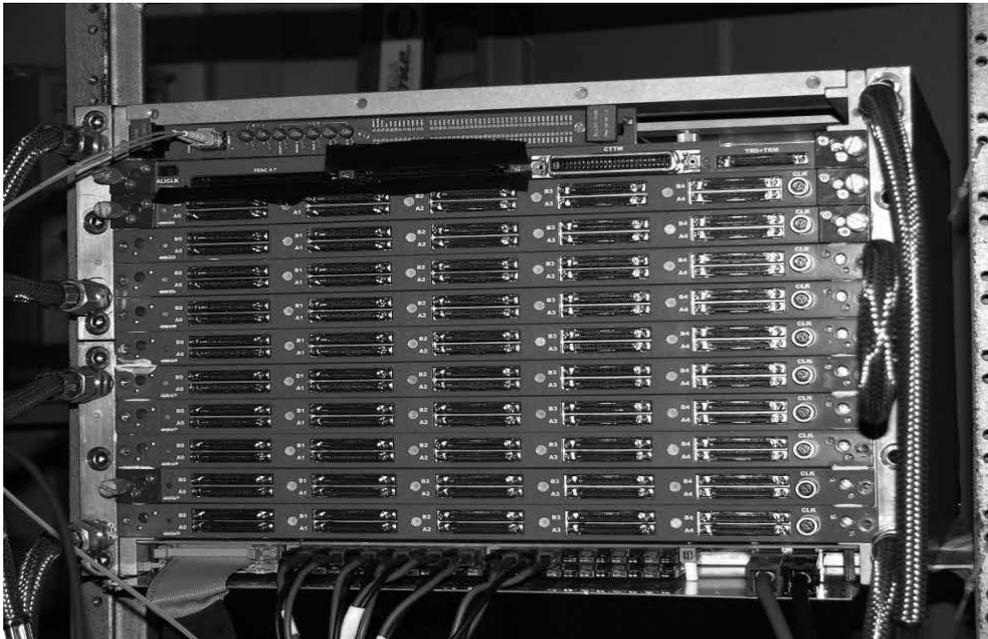
**Figure 7:** Custom VME crate with the readout electronics used in the ALICE TOF system.
