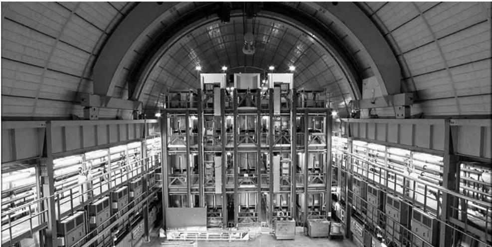
**Figure 2:** The Large Volume Detector at LNGS. The liquid scintillator is contained in the blue tanks.
